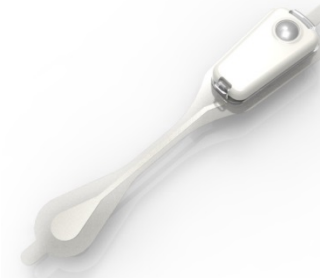
Sternal location of the CAM monitor and electrode spacing gives a hybrid ECG of V1 + aVF.
